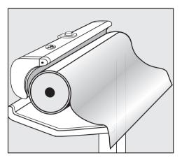
Completely unwind the cotton undercloth attached to the roller and let it hang down smoothly.
