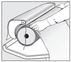
Insert the raw edge of the new ironing cloth into the retaining slot with the wrong side down. Leave the cords hanging free and smooth out the cloth.
