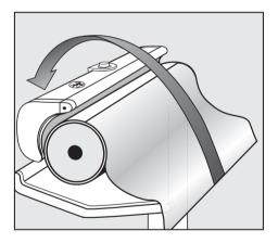
Take hold of the cloth by each side edge and keeping it taut place over the heater plate.
