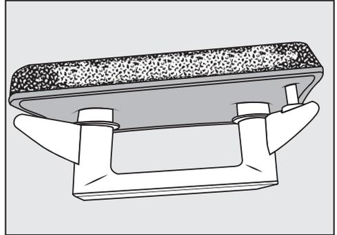
Residues arise from laundry fibres and traces of detergent components. They can be found on the front and side edges of the plinth filter. In extreme cases, they can form stubborn crust. Residues are a sign that the plinth filter no is longer a snug fit at the sides, even if it appears to be perfect: lint is getting in unfiltered at the edges.
