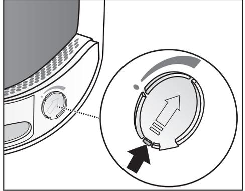
If you are not using a fragrance capsule: push the tab down completely (see arrow) so that the socket is closed. Otherwise, lint will accumulate here.
