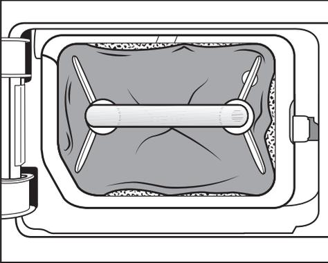
The edges of the plinth filter do not sit properly and the plinth filter is deformed. Lint will blow into the heat exchanger unfiltered through edges that do not sit properly. This will cause a permanent obstruction in the heat exchanger.
