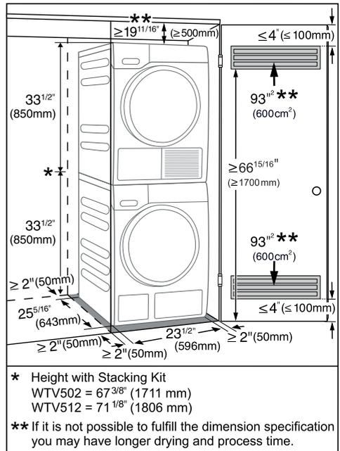
⚠ Ensure that the dryer door can be opened at any time. Ensure that the laundry can be removed at any time without hindrance.
