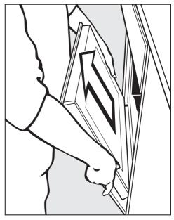
■ Hold the door on either side and pull it diagonally upwards off the retainers. Make sure that the door goes back on straight.
