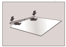
■ Secure the profiled seal to the middle glass pane.
