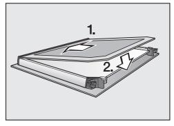
■ Push the inner pane with the matt printed side facing downwards into the plastic strip and place it between the retainers.
