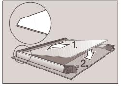
■ Then refit the middle glass pane together with the profiled seal.
