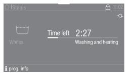
**Tip:** You can use the pull-down menu to display the selected temperature, spin speed and any selected Extras.
