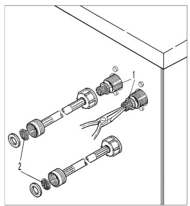
■ The filters in the water intake valves (1) and the inlet hoses (2) must be checked for contamination from time to time and cleaned as necessary.
