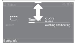
If an orange bar appears at the top of the screen in the middle of the display, you can open the pull-down menu. Drag the bar downwards to display it. To hide it, slide the bar upwards again.
