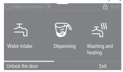
The individual functions of the machine can be selected individually and the parameters can be set.
