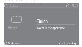
The suds are not drained so they can be used again in a subsequent programme. Once the programme has ended, the programme end screen is displayed. It is possible to switch to the main menu while the suds are in the drum or to drain the suds by pressing the Start draining control. If permanent automatic water drainage is required, Automatic drainage can be activated at supervisor level.
