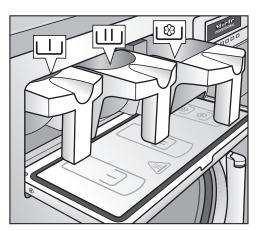
■ For standard wash programmes add the powder detergent for the main wash to the Ш drawer and if desired, add detergent for a prewash to the U drawer. Add fabric conditioner to the front of the drawer.
