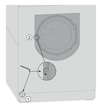
■ Using a T 40 Torx wrench, turn the release element with the inner hexagon ② two whole revolutions anti-clockwise.
