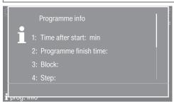
Once the delay start period has elapsed (if applied), the programme running time will appear in the display; otherwise, the running time will appear straight away. The programme sequence is also shown in the display.
