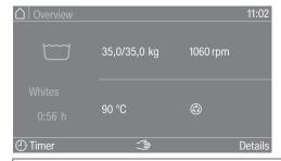
The Boost Spin function cannot be selected or deselected in the Extra sub-menu. The symbol is displayed in a different colour.
