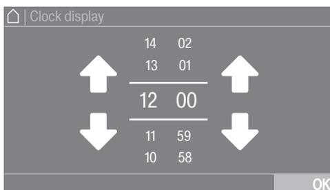
Enter the numbers by swiping upwards or downwards. Place your finger on the number that you want to change and move your finger in the direction you want. Use the OK sensor to accept all set figures.
