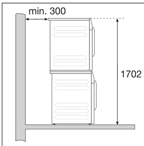
A stacking kit\* is required. This must be fitted by a Miele authorised technician.
