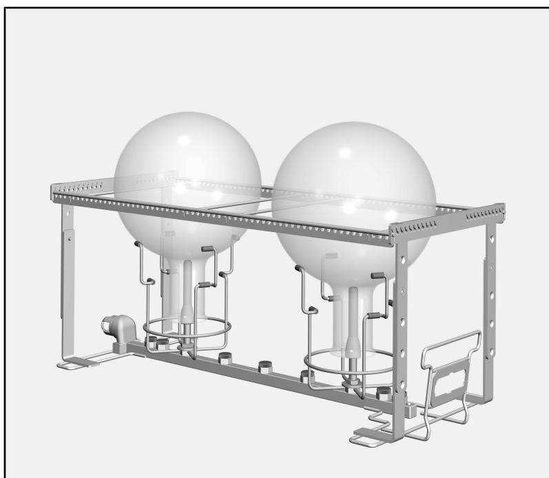
The round flasks rest on 4 points of the support; their necks should not touch the water supply pipe.
