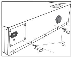
■ Remove the safety screws ④ from the back of the drawer.
