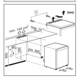
If your appliance is supplied with wall spacers, these must not be used if the appliance lid has been removed (see "Installation – Location").
