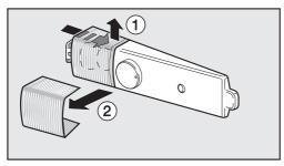
Reach the back of the lamp cover, press up at the sides ①, and pull the lamp cover ② off.
