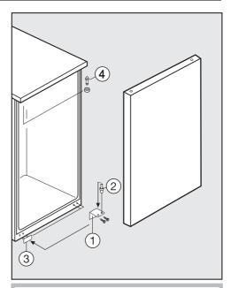
Danger of injury when removing the appliance door. The appliance door is not secure once the screws on the hinge bracket have been removed. Hold the appliance door firmly.
