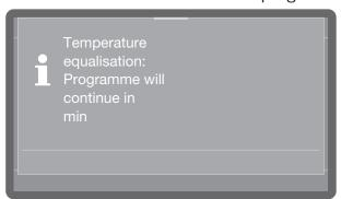
If the temperature inside the wash cabinet is more than 60 °C at this point, the pressure is equalised first. Then the programme continues.
