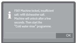
■ Follow the instructions on the display and top up the reactivation salt, see i "Filling the container for reactivation salt".
