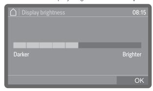
■ Adjust the brightness of the display and press *OK* to save the setting.
