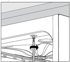
■ Remove the cover caps on the left and right. Screw the machine to the continuous worktop through the holes in the front trim. Then refit the cover caps.
