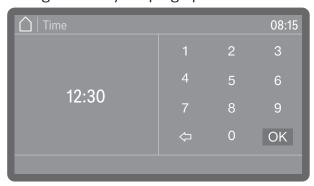
Secondly, you can call up a numerical keypad by briefly tapping the numbers highlighted in colour and then entering the numbers directly.
