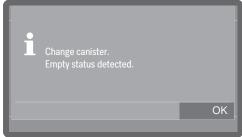
System messages are indicated by the information symbol 1. These give information about current processes and the status of the machine. If there is more than one system message, they are shown one after the other and — depending on the message — must be processed or acknowledged individually.
