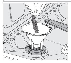
■ Place the salt funnel on the refilling opening.
