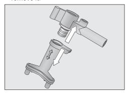
Release the upper section with the holder for the milk pipework from the dispensing spouts.
