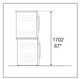
A stacking kit\* is required. This must be installed by a service technician authorized by Miele.
