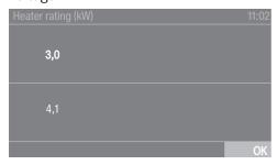
208 V  $\rightarrow$  3.0 kW heater rating 240 V  $\rightarrow$  4.1 kW heater rating
