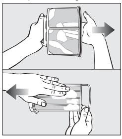
Use your fingers or a vacuum cleaner to remove the lint from the surface of the filter.
