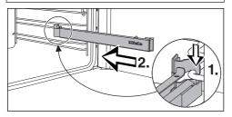
Hook the FlexiClip runner onto the front of the lower rail of a shelf level (1.) and then push it along the rail into the oven compartment (2.).
