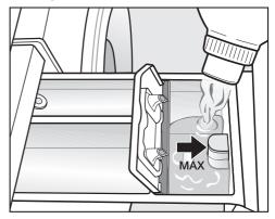
■ Add fabric softener or liquid starch to the ※ compartment. **Do not exceed the maximum level mark.**
