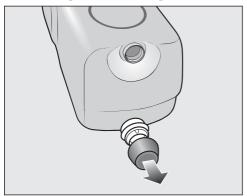
Remove the cover cap from the cartridge.
