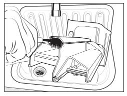
Clean the fabric softener channel using a brush and warm water.
