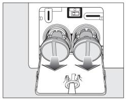
■ Remove the filters completely.
