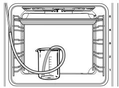
Place the container with the descaling solution on the floor of the oven compartment.
