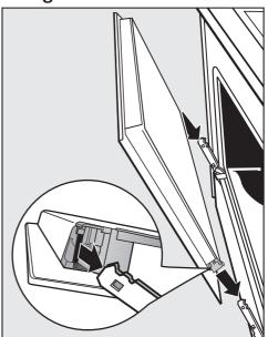
■ Hold the door securely on both sides and carefully fit it back into the hinge retainers.
