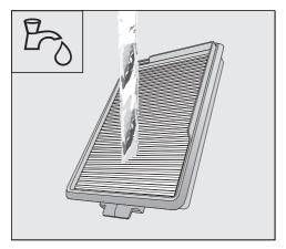
■ Rinse the pleated side of the fine dust filter under cold running water.
