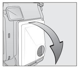
■ Remove the fine dust filter in the direction of the arrow.
