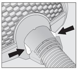
If you want to separate the pieces again, press the release catches at the side of the hose connector, and pull the suction hose out of the suction opening.
