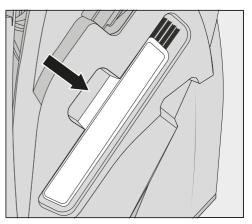
■ Take the cleaning tool out of the side flap on the dust container.
