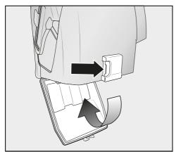
■ Press the release catch on the bottom of the dust container.
