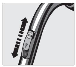
Open the air inlet valve on the handle far enough to reduce the suction power.
