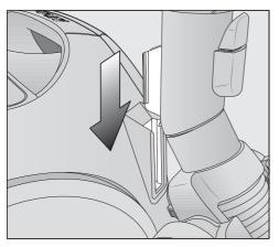
Slot the floorhead or floorbrush into the park system from above.
