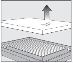
■ Remove the filter mat from the fine dust filter.
