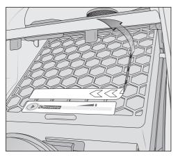
■ Remove the indicator strip from the HEPA AirClean exhaust filter.
