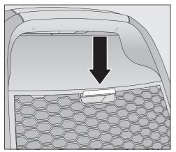
Press the release catch on the exhaust filter compartment flap and remove the flap.
