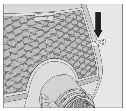
You will recognise that the HEPA AirClean exhaust filter is fitted to the appliance by an indicator strip hanging out of the exhaust filter compartment.
