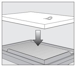
■ Attach the dry filter mat to the dry fine dust filter so that the soft side of the filter mat is pointing up and the loop used to remove it is visible.
