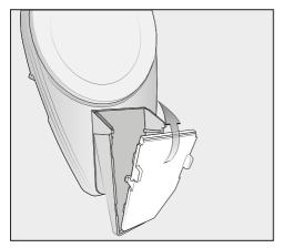
Refit the filter at the bottom of the dry filter frame and close it, making sure it clicks into position.
