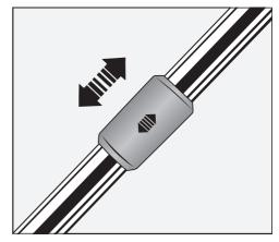
Grasp the release mechanism and adjust the telescopic suction tube to the required length.
