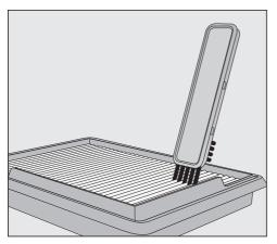
Clean the pleated side of the fine dust filter with the long brushes on the cleaning tool.
