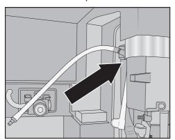
Connect the angular moulded hose to the longer milk pipework. Start by fitting the moulded hose to the top of the central spout. The black connecting piece should point towards the rear.
