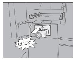
■ Fit the holder with the silicone seal until it clicks into position.
