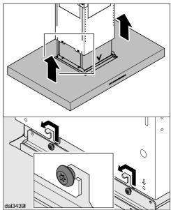
■ Hang the rangehood on the brackets, making sure that the controls are at the front.
