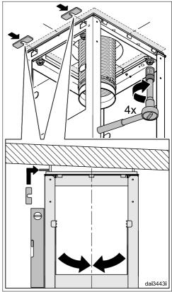
Align the installation frame and secure it with the screws. The spacers, which were removed from the spacer frame at the start, can be used to align the rangehood vertically.
