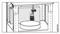
The strain relief must be used to ensure problem-free connection.
