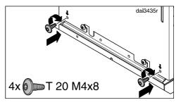
■ Secure the rangehood with the screws supplied.
