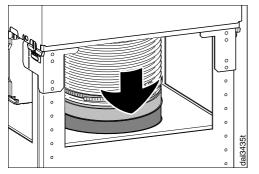
Place the exhaust ducting onto the exhaust socket.
