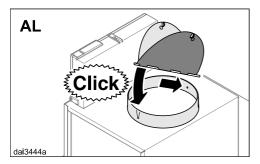
■ With extraction mode (AL), fit the non-return flap in the exhaust socket if your ducting system is not equipped with one.
