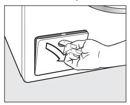
■ Open the drain pump access panel.
