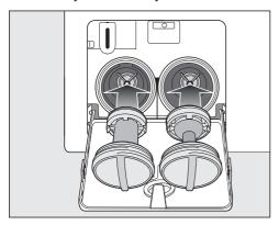
Replace the drain filters correctly (on the right and left) and tighten them securely. Risk of damage from leaking water.
