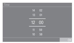
Enter the numbers by swiping up or down. Place your finger on the number that you want to change and move your finger in the direction you want. Use the *OK* sensor control to accept the set numerical value.
