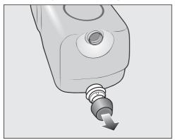
Remove the cover cap from the cartridge.
