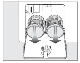
■ Remove the drain filters completely.
