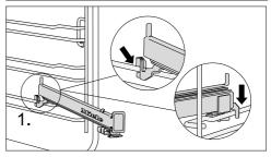
■ Hook the FlexiClip runner onto the front of the top rail of a side runner (1.).
