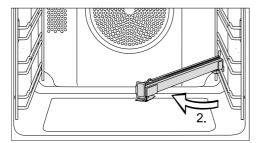
■ Then hold the FlexiClip runner at an angle towards the middle of the oven compartment (2.).
