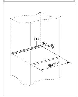
■ Create a cut-out ① in the intermediate shelf where the steam combination oven is to be placed.
