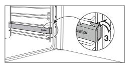
■ Then secure the FlexiClip telescopic runner to the lower rail of the shelf level as illustrated (3.).
