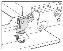
■ To relock the locking clamps, flip them back up to the horizontal position as far as they will go.
