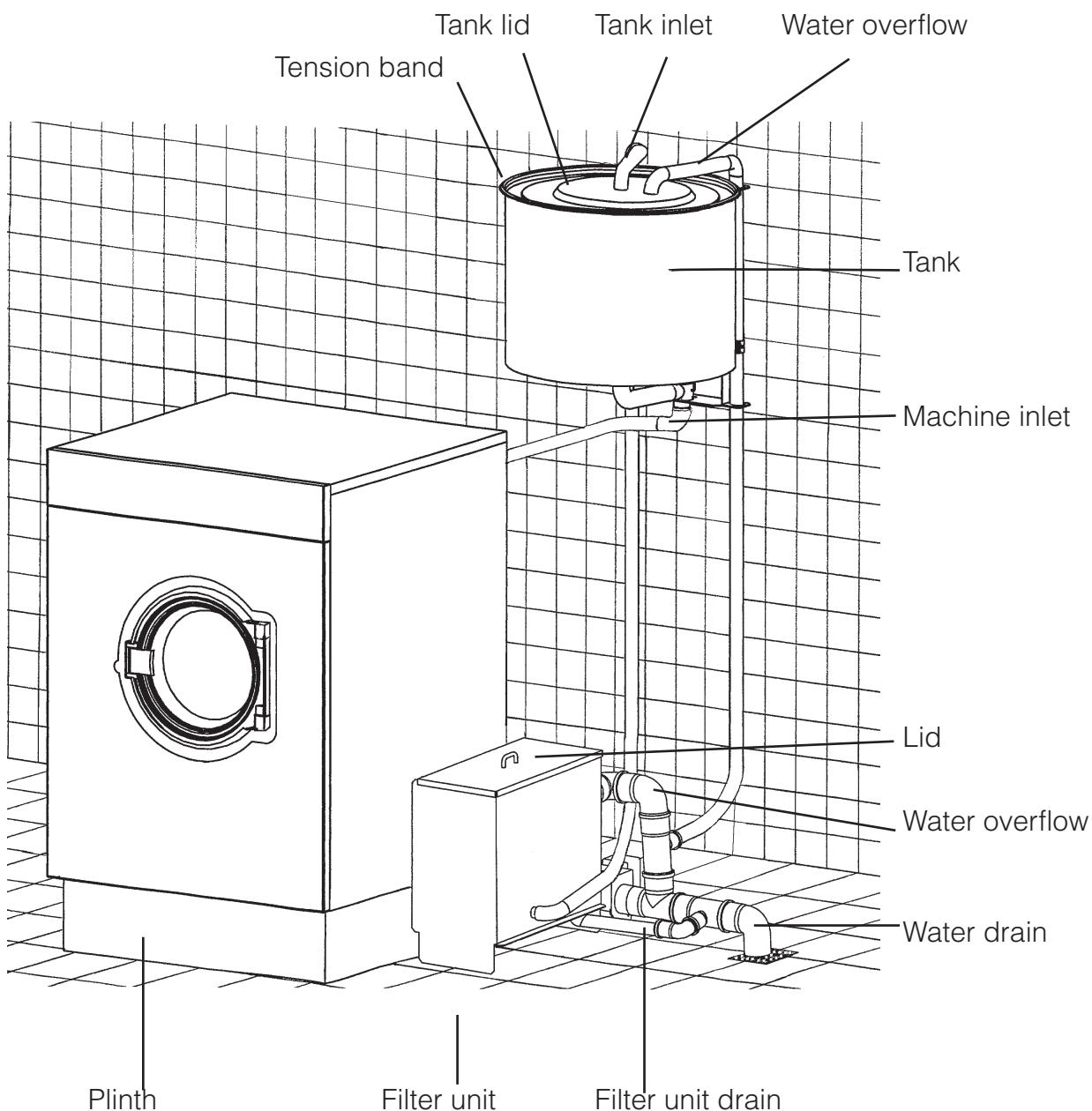
The water recycling unit "WRG" must only be installed by an approved Service technician or authorized Service Dealer.
