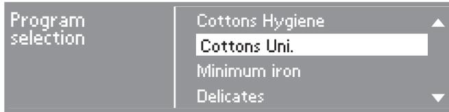
All programs can be selected with the jog shuttle. Depending on the direction the jog shuttle is turned the highlighter moves up or down.
