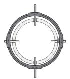
Place the wok ring on the pan support so that it sits securely in position and cannot move (see diagram).
