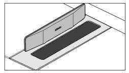
Install the FlameGuard directly next to the downdraft extractor when you are operating a gas cooking element.
