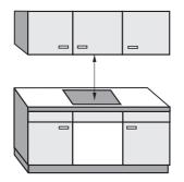
The safety distance specified by the manufacturer of the cooker hood must be maintained between the SmartLine element and the cooker hood above it.
