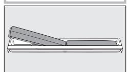
Remove both charcoal filters and place the new filters with the surrounding edge pointing downwards in the holder.
