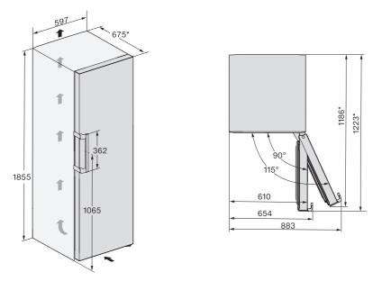
$\star$  Dimensions without wall spacers fitted. Appliance depth is increased by 15 mm with the supplied wall spacers fitted.
