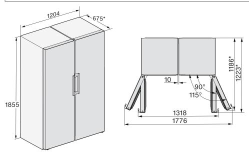
$^{\ast}$  Dimensions without wall spacers fitted. Fitting the wall spacers supplied increases the appliance depth by 15 mm.
