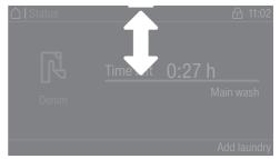
If an orange bar appears at the top of the screen in the middle of the display, you can open the pull-down menu. Touch the bar and drag down with your finger.
