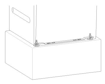
The anchors provided can be used to bolt the machine to the floor by both front feet. The fasteners provided are intended for use in bolting the machine to a concrete floor.
