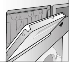
If the drip channel and its drain connector are blocked, then these should be cleaned.
