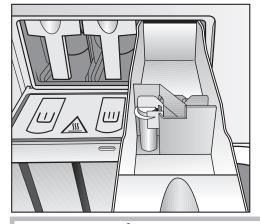
Do not fill the  $\$  compartments above the level marker with liquid agents.
