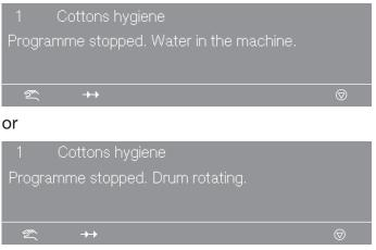
**Useful tip:** To open the door, select the "Water drainage" t<sub>⊥</sub> button or select the "Separate spin" programme and press "START".
