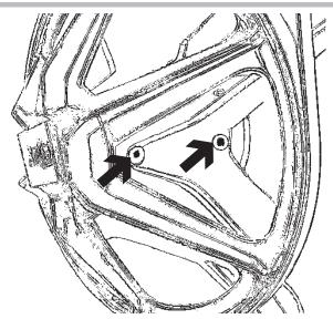
Lubricate the drum shaft bearings after approx. 1000 operating hours via grease nipples with Arcanol L 100 grease.
