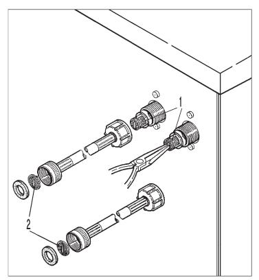
The filters in the water inlet valves (1) and the inlet hoses (2) must be checked for soiling from time to time and cleaned if necessary.
