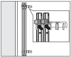
Secure the transit bars to the back of the washing machine. Make sure that the top catch is located above the holder. Risk of damage from incorrect transport.
