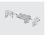
■ Disassemble the dispensing unit into
