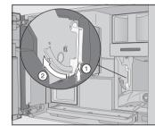
■ Press the button under the handle of the brew unit 1 and, while doing so, turn the handle forward 2.
