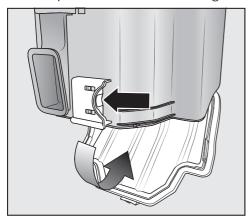
■ Press the yellow release catch on the bottom of the dust container.
