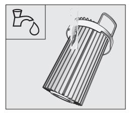
■ Rinse the outside of the fine dust filter under cold running water.
