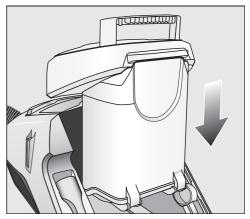
Insert the dust container into the vacuum cleaner from above so that it audibly clicks into place.
