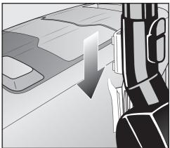
Slot the floorhead or floorbrush into the parking attachment on the vacuum cleaner.
