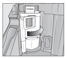
Release the fine dust container from the vacuum cleaner in the direction of the arrow and remove it.
