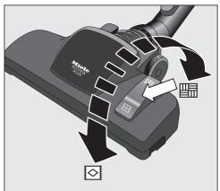
Clean even hard floors which are not susceptible to scratching, as well as flooring with gaps or deep crevices in it with the brush protruding:
