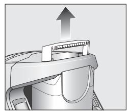
Pull the dust container handle upwards.
