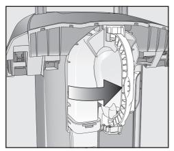
■ Release the handle of the pre-filter and remove the pre-filter.
