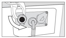
Unscrew the stopper from the hot water valve.
