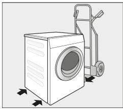
If transporting the washing machine with a hand trolley, make sure only its left or right side is resting on the trolley.
