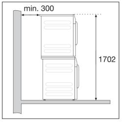
This washing machine can be installed with a Miele tumble dryer on top of it. This requires a Miele washer-dryer stacking kit which can be purchased separately. A Installing the washer-dryer stack on a Miele plinth is not permitted.
