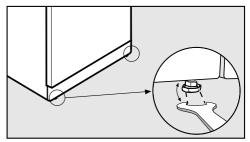
■ To align the refrigeration appliance, adjust the front feet using the open spanner.
