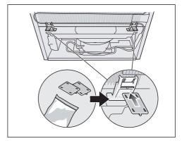
■ Slide the provided wall spacers into the holders on the left and right of the rear appliance panel.
