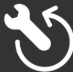
The warewasher control unit specifies the number of operating hours or wash cycles at which the pictogram for service is shown.
