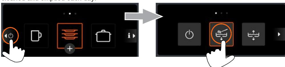
Pressing the On/Off button switches the warewasher off. The tank stays filled but will no longer be kept at temperature. If the tank temperature has dropped too much before the machine is switched on again, the machine will be emptied and refilled automatically.
