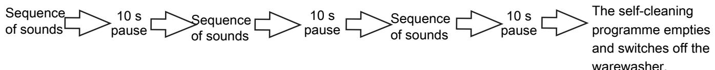
If the door is open during the automatic switch-off, the warewasher is pumped empty and switched off, but is not cleaned on the inside.
