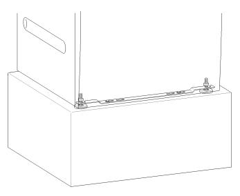
The anchors provided can be used to bolt the machine to the floor by both front feet. The material provided is intended for use in bolting the machine to a concrete floor.
