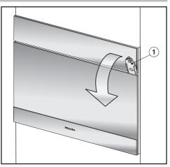
■ Insert the door tool ① supplied about 1 1/2" (3 cm) into the gap between the door and the control panel on the right-hand side and then pull the door open.
