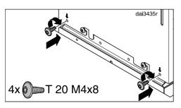
Secure the rangehood with the screws supplied.
