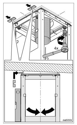
Align the installation frame and secure it with the screws. The spacers, which were removed from the spacer frame at the start, can be used to align the rangehood vertically.
