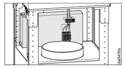
The strain relief must be used to ensure problem-free connection.
