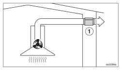
In extraction mode the silencer not only reduces noise from the fan outside the house, but also sounds from outside which reach the kitchen via the vent ducting (e.g. traffic noise). For this reason, the silencer must be positioned as close as possible to the ducting exit (1).
