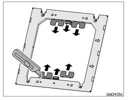
Use a knife to release the four spacers and the two covers from the spacer frame supplied.
