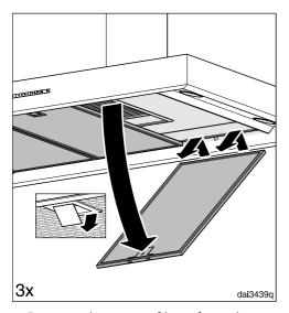
■ Remove the grease filters from the rangehood.
