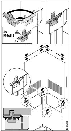
■ Fit the four telescopic piece clamps. When the screws are tightened, the clamps spread out and push the telescopic piece upwards.
