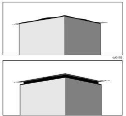
The **spacer frame** can be installed between the tower and the ceiling. This creates a shadow which gives the illusion of a gap between the ceiling and the tower. This is useful if the ceiling is not level or is uneven. The rangehood is aligned vertically with the spacers supplied. Visual irregularities between the tower and the ceiling are then concealed by the shadow.
