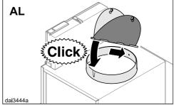
■ With extraction mode (AL), fit the nonreturn flap in the exhaust socket if your ducting system is not equipped with one. Recirculation mode (UL) does not require the non-return flap to be fitted. If there is one present, it should be removed.
