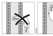
If the exhaust air is to be ducted into a vent flue, the ducting must be directed in the flow direction of the flue.
