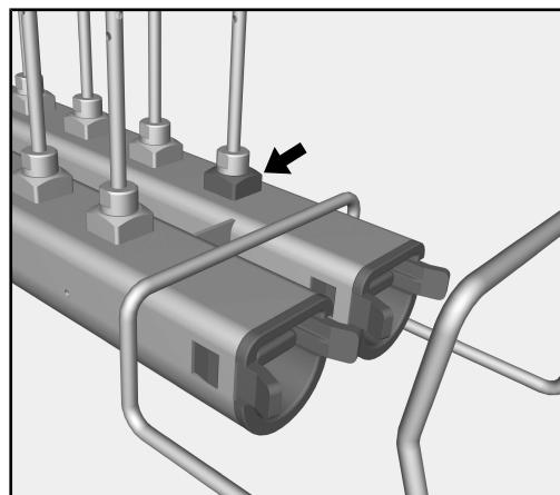
The holder at the top of the right-hand injector rail is used as the test point for measuring water pressure. This connection point can be used for testing wash pressure within the framework of performance and validation testing in accordance with EN ISO 15883.
