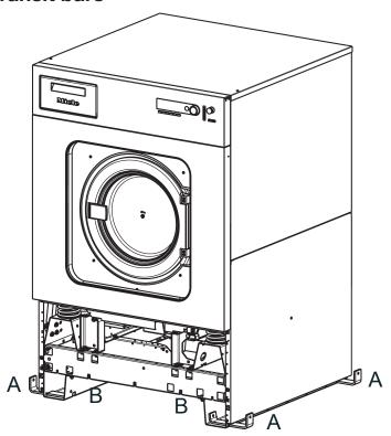
The fastening brackets "A" on the sides, 2 each on the left and right, for the transport crate are each fastened with one hexagon head screw and can be removed.
