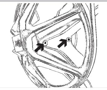
Use grease nipples to lubricate the drum shaft bearings with Arcanol L 100 grease after approx. 1000 operating hours.
