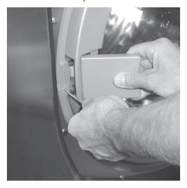
■ First insert the screwdriver into the opening next to the door lock, press it in and hold it. Press against the door handle with your right hand and then pull the door handle to open the drum door. Never use force to open the drum door!
