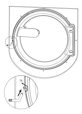
■ Using a T 40 Torx wrench, turn the release element with the inner hexagon 2 whole revolutions in the direction of the arrow.
