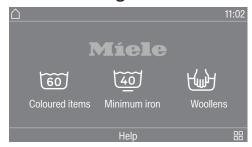
Up to 24 preset programmes are available. The first 3 programmes can be selected directly. The remaining programmes are selected from a list 品. These programmes cannot be changed by the operator.
