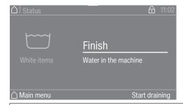
The suds are not drained so that they can be further used in a subsequent programme. After the programme has finished, the display for the programme end mask/programme end screen will appear. It is possible to change to the main menu with the suds in the machine or drain the suds by pressing the Start draining selection field. If permanent automatic water drainage is required, Automatic drainage can be activated at supervisor level.
