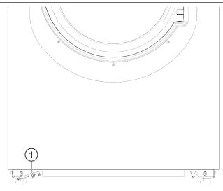
■ Guide the T 40 Torx wrench for the emergency door release through the eye ① on the front of the machine.
