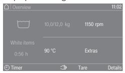
■ If after resetting to O (taring), you remove an overlooked item from the drum, the following will appear in the display:
