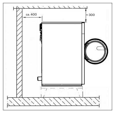
Minimum distance to the wall approx. 400 mm to allow for maintenance.
