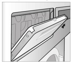
If the drip channel and its drain connector are blocked, then these should be cleaned.
