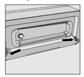
Insert the plug of the supplied power supply unit into the socket at the back of the base station. You can wind excess cable around the cable rewind. Guide the cable through one of the two cable guides.
