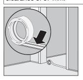
Place the magnetic strip supplied with the groove facing downwards on the floor.
