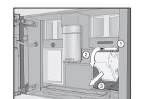
■ Pull the brew unit sideways ① and tilt it forwards 2. Pull the brew unit forwards to remove it 3.
