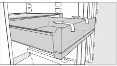
Pull the drawer out as far as it will go. Tilt the drawer up slightly and remove the drawer.
