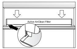
Place the holder in the middle of the protective strip at the back of the adjustable shelf so that it clicks into position.  Touch the symbol on the display to confirm that the filters have been replaced.
