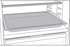
Place the baking tray on the adapters in the refrigerator section and slide it in as far as it will go.
