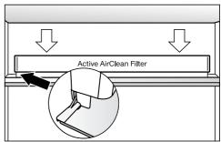
Reinstall the holder on the protective strip.
