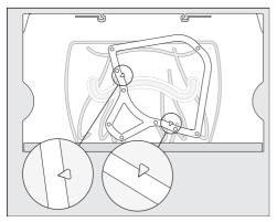
Place the frame on the adjustable shelf so that the arrows on the adjustable shelf line up with the recesses on the frame.
