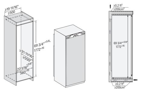
\* The declared energy consumption was achieved with a niche depth of 22 1/16" (560 mm). The refrigeration appliance is fully capable of functioning at a niche depth of 21 5/8" (550 mm) but will consume slightly more energy. Before installation, ensure the housing-unit dimensions are the correct size.
