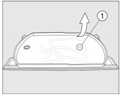
Take a firm hold of the top right of the bottom adjustable shelf and pull the tray firmly off the adjustable shelf.
