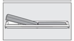
Remove both charcoal filters and place the new filters with the surrounding edge pointing downward in the holder.
