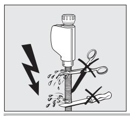
① Do **not** shorten or otherwise damage the inlet hoses supplied with the machine.
