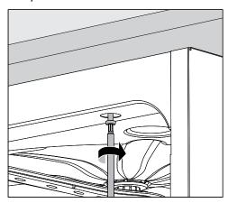
■ Screw the machine to the continuous countertop through the holes in the front trim on the left and right.
