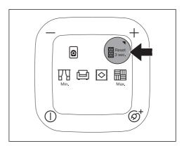
You must reset the indicator each time you replace the exhaust filter. The vacuum cleaner must be switched on to do this.
