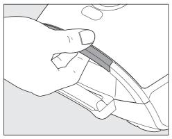
Press the release button in the recessed grip for the dust compartment lid and raise the lid as far as it will go.
