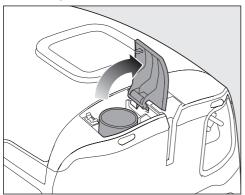
■ Press the release button on the accessories compartment.
