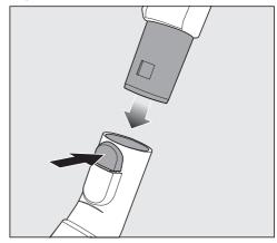
Push the suction tube into the floorhead and turn it clockwise or anti-clockwise until it clicks into position. ■ To separate the suction tube from the floorhead, press the release button and pull the suction tube away from the floorhead, twisting it slightly as you do so.
