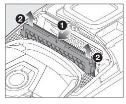
If you wish to fit an AirClean exhaust filter, see "Replacing one type of exhaust filter with another".
