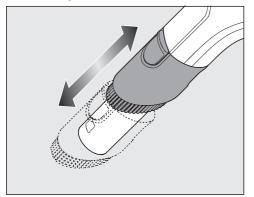
■ Press the release button on the dusting brush and push the brush out until it clearly engages in position.
