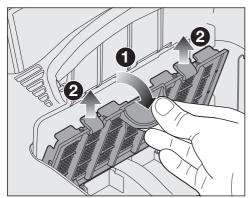
Release the motor protection filter forwards and remove it upwards from the dust compartment.
