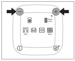
Press the + foot switch to select a higher suction power level. Press the - foot switch to select a lower suction power level.
