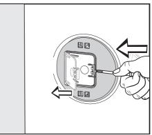
Press against the retainer with a sharp object (a narrow screwdriver, for example).
