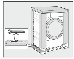
Take out the open spanner for removing the transit bars from the bottom left of the transport packaging.
