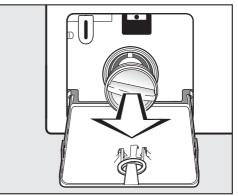
■ Remove the drain filter completely.
