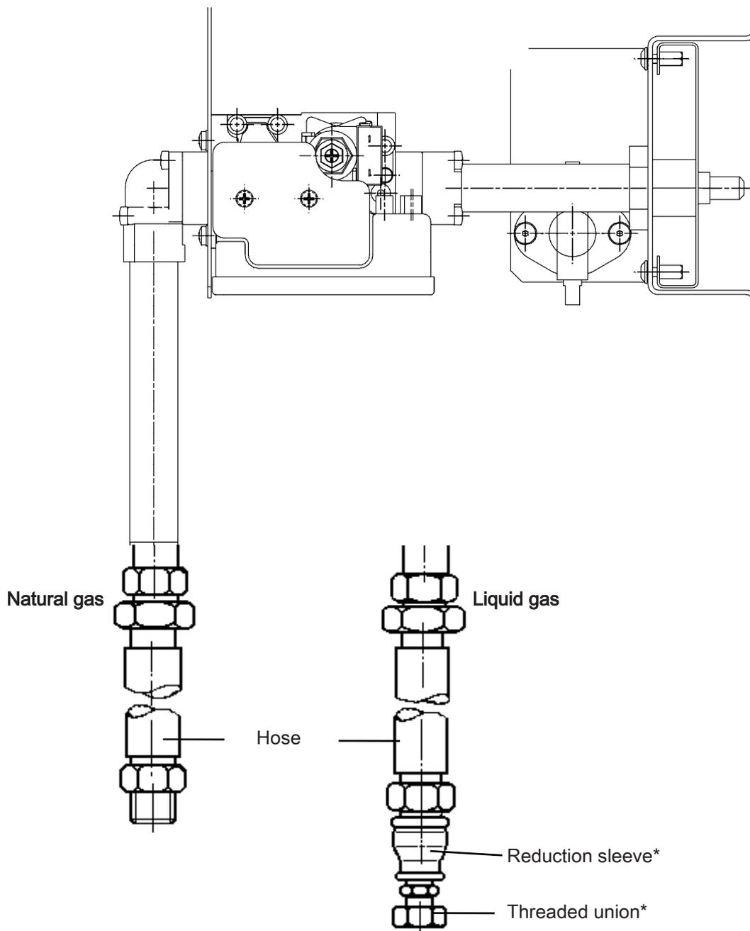
\* Supplied with the conversion kit for natural gas to liquid gas.
