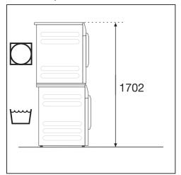
The washing machine can be installed as a washer-dryer stack together with a Miele tumble dryer. This requires a Miele washer-dryer stacking kit which can be purchased separately.
