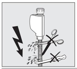
⚠ Do **not** shorten or otherwise damage the water inlet hoses supplied with the machine.
