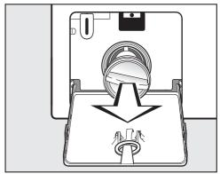
Remove the drain filter completely.
